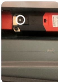
Left: The interlock guard switch unit (circled) is located behind the lower front machine panel.
